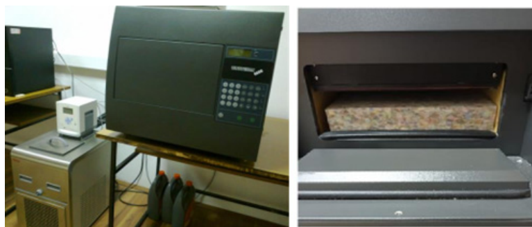
Figure 1: Heat Flow Meter: a) instrument configuration, b) sample placed in the HFM instrument.
