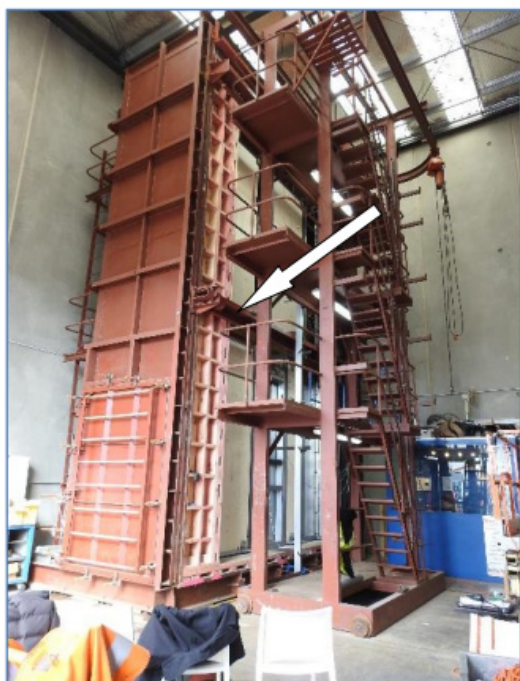
Figure 5: Inter-storey racking test of a curtainwall prototype.
