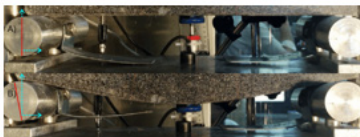
Figure 39: Looseness of the right-side support along with an eccentric rotation during the FPBT; A) before loading the specimen, and B) after loading the specimen.
