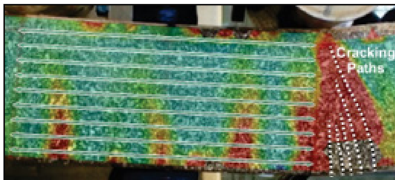
Figure 25: Formation of the cracks at the shear-span for the third specimen of the mixing proportion MS-30 at the MOR stage.
