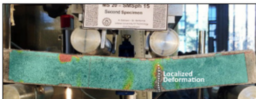
Figure 21: Localized deformation at a single crack after the MOR stage for the second specimen of the mixing proportion A-15.
