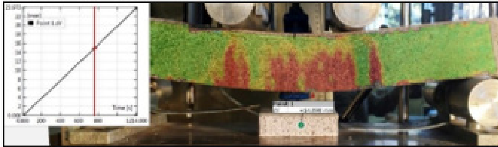
Figure 8: Speckled pattern placed on the loading deck and the calculated displacement data during the test for the specified point on the pattern.
