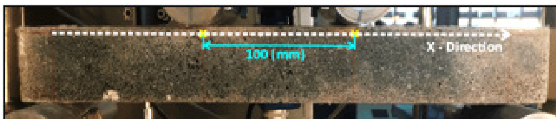
Figure 7: The marked line and the specified distance on the specimen surface, indicating the x-direction and the distance computational reference, respectively, in the DIC software.
