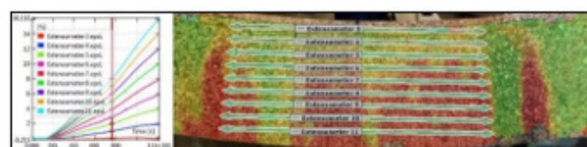
Figure 11: The calculated longitudinal strains data during FPBT for the virtual extensometers on the surface of the bending beam.
