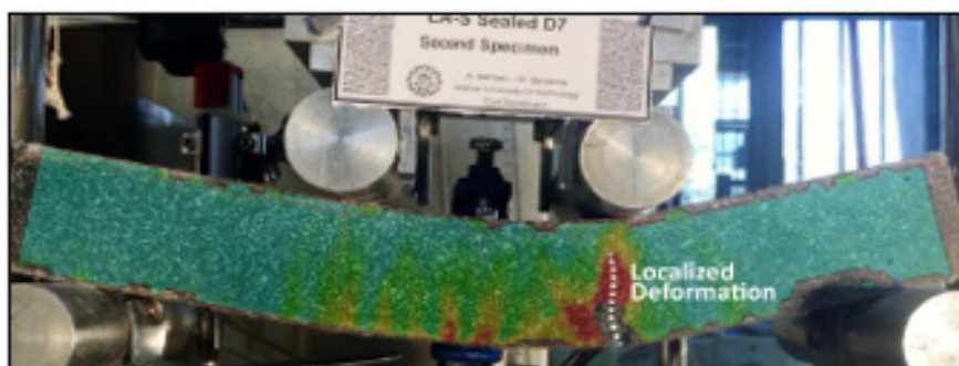
Figure 20: Localized deformation at a single crack after the MOR stage for the second specimen of the mixing proportion LAS-D7.
