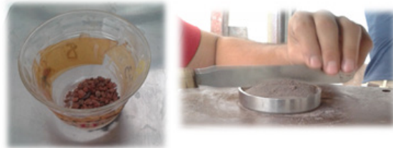
Figure 1: Natural void structures (scoria), expansive soil and consolidation ring.
