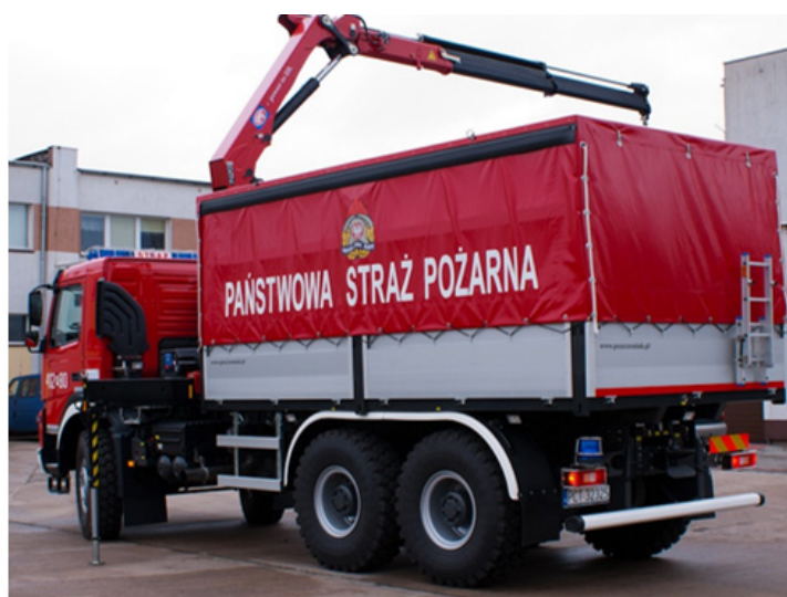
Figure 13: An example of a truck with an HDS device (Volvo FMX 66R 420 6x6, JRG Trzcianka, Poland). Source: www.czerwonesamochody.com (photo: Maciej Chmielewski)
