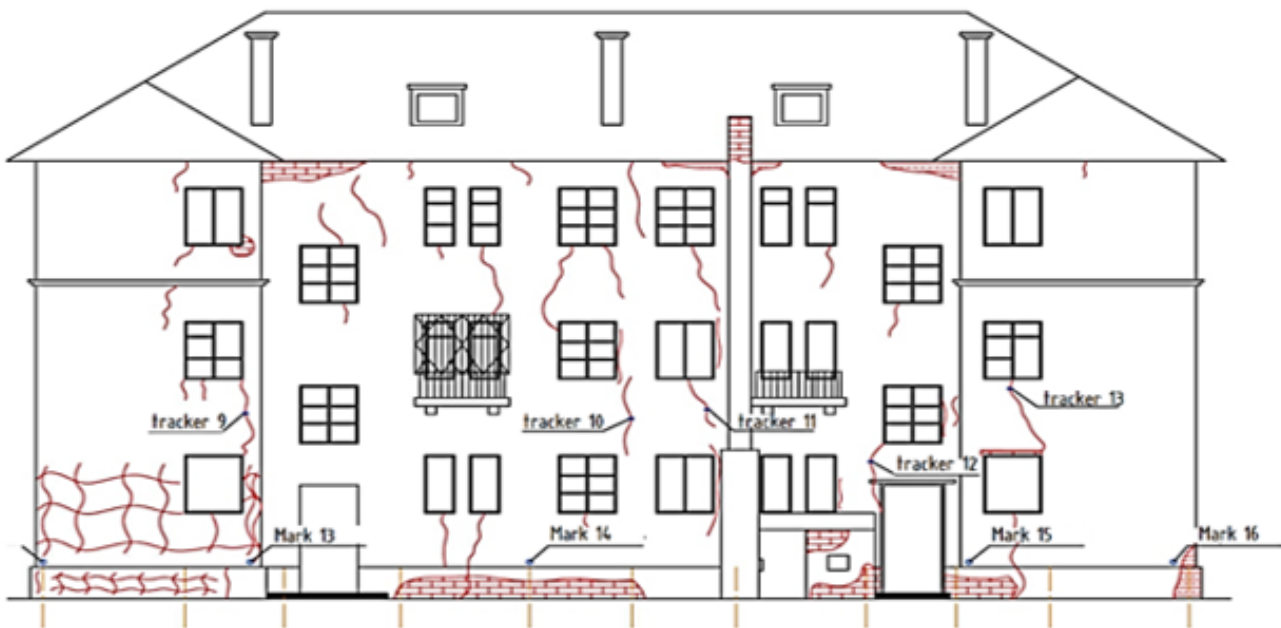
Figure 3: Front facade of the five-story apartment building with indication of deformation cracks.
