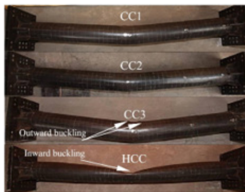
Figure 56: Failure modes of the outer steel tube of the experimentally tested specimens after impact by Han et al. [111].
