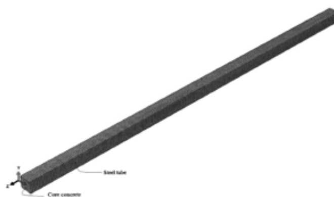
Figure 46: Numerical model of concrete-encased concrete-filled steel tube (CFST) by Yousuf et al. [107].
