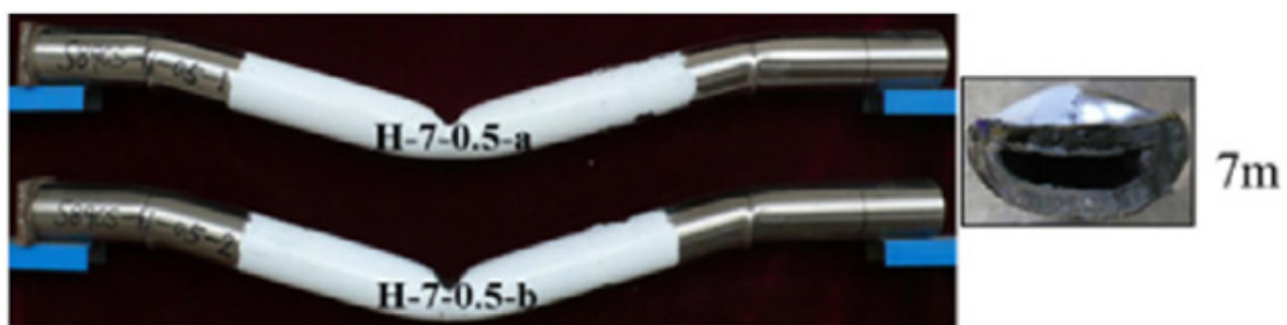
Figure 97: Specimen with tag number H-7-0.5-b which had the highest impact time and the highest residual displacement after impact load among all researchers by Zhao et al. [84].
