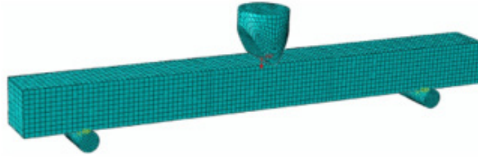
Figure 52: Numerical model of HSCFST subjected to transverse impact by Yang et al. [169].
