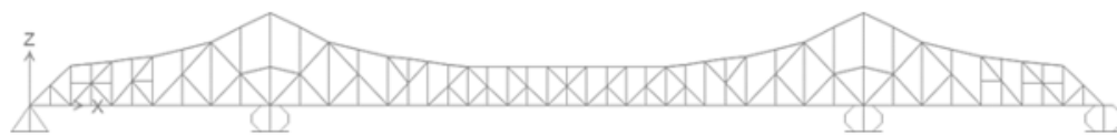
Figure 3: Finite element model for the as-built main system of the steel bridge.
