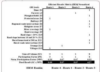
Figure 2: Screenshot from SIMUS last screen with result with data from GIS.
