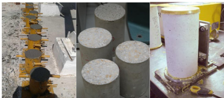
Figure 1: Compressive strength test. (a): Preparation of cylindrical specimens 16 x 32 cm; (b): Specimens removed from the molds; (c) surfacing of cylindrical specimens with sulphur
