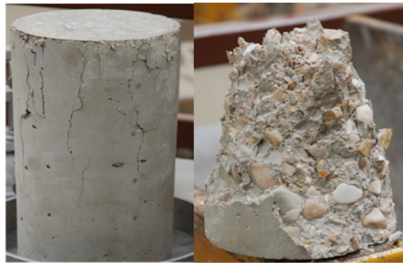
Figure 6: Compressive strength test. (a) Appearance of cracks in the lateral surfaces of the test specimen due to tensile stresses; (b) : Conical rupture of the specimen.
