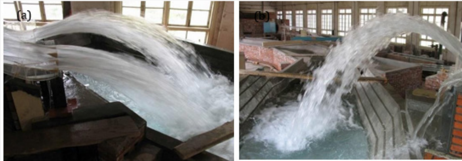
Figure 3: The physical model of flow pattern over two types of spillway crest.
