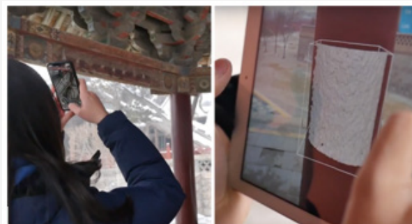
Figure 3: Capturing weathered column surface and internal space with Structure Sensor 3D Scanner (right) & Display Land application (left).
