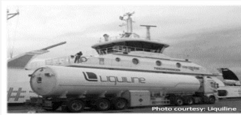
Figure 9: Truck as a Facility for Transferring LNG to Vessel [42].
