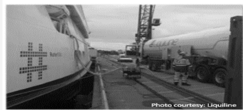
Figure 10: Truck as a Facility for Transferring LNG to Vessel [42].
