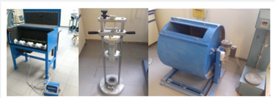
Figure 4: Micro-Deval, AIV and Los Angeles Device (Laboratory of Engineering Geology, Patras University).
