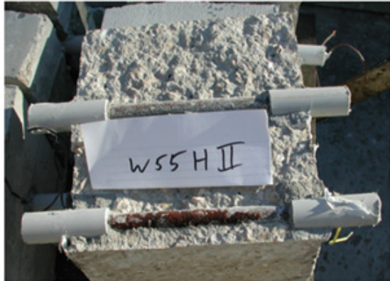
Figure 4: Split specimen a few months after corrosion initiation.
