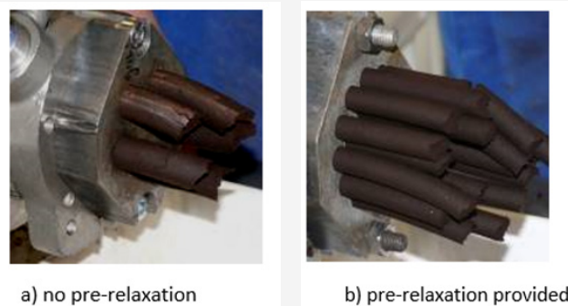
Figure 3: Pellet molding process.
