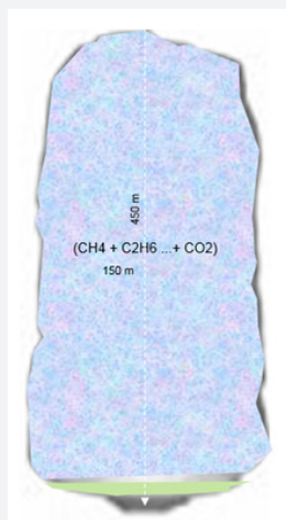
Figure 29: Abandonment of the cavern filled with gases.
