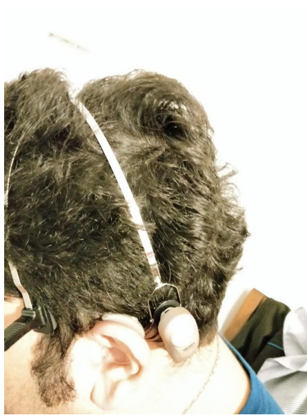
Image A: Receiver in the Ear Hearing Aid and Bone conduction Hearing Aid at the same time.
