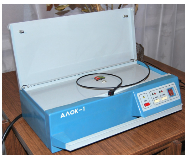
Figure 1. Helium-neon laser -Alok-1, wavelength 632.8 nm, 1-2 mW.
