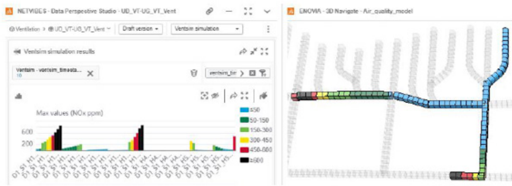
(a) Visualised AQ simulation results in the VT app: Ventsim (NO x ppm) at t = 10 min.
