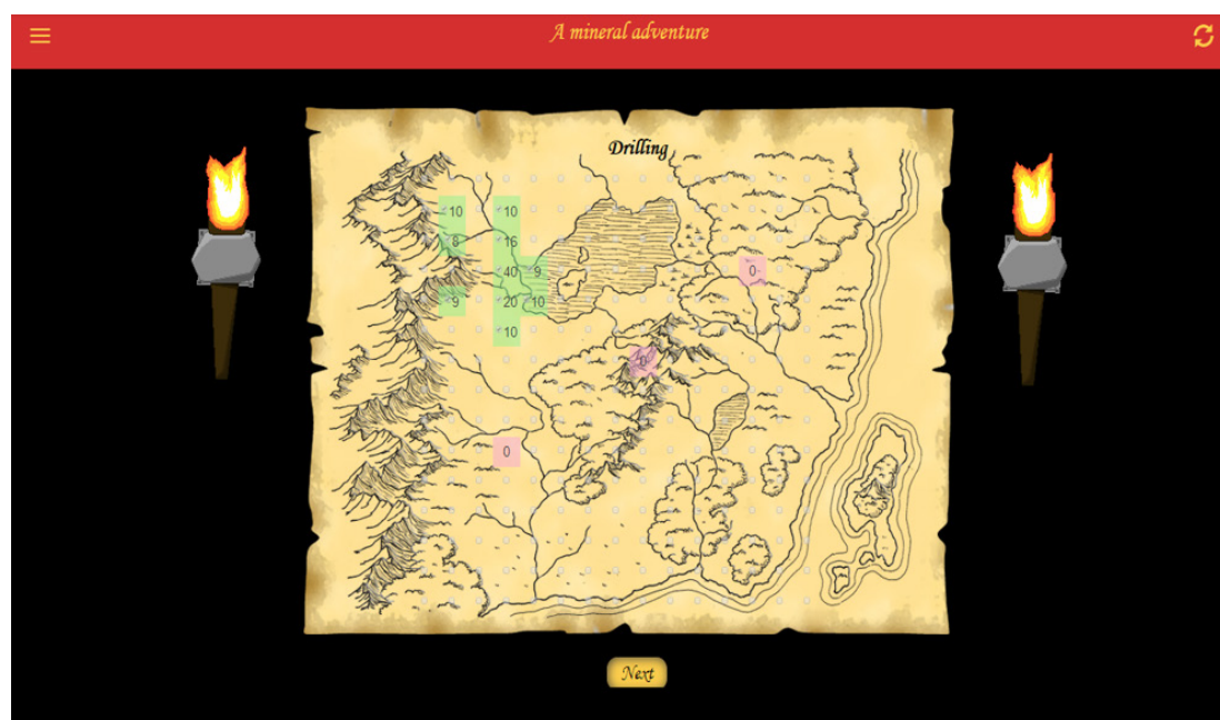
Figure 1: Map of the area to be explored, after conduction of a drilling campaign: green colored blocks indicate orebody existence and pink colored blocks indicate zero ore ingredient.
