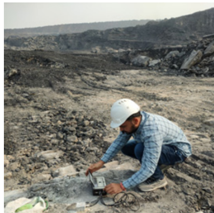
Figure 3: Installation of Mini-Seis III for measuring vibrations.
