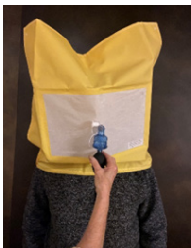
Figure 3: Fit test chamber to see if seal of mask is satisfactory.
