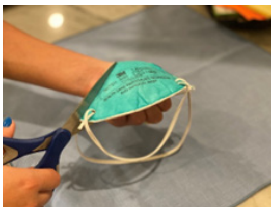
Figure 1: The N-95 coincidentally has a horizontal crease at the equator that allows for an easy bisection into two halves that are almost equal in size.
