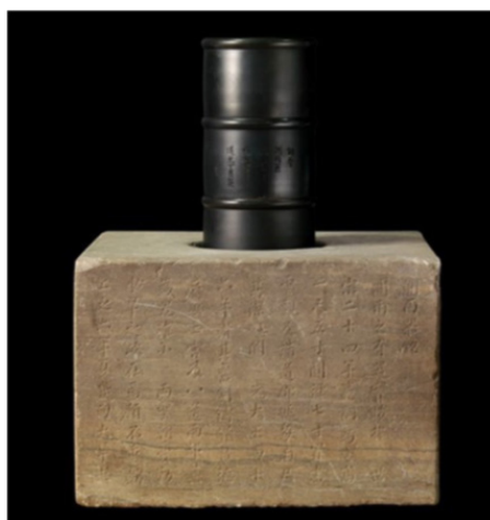
Figure 1: Cheugugi, the world's oldest rain gauge devised in the Joseon Dynasty in 1441. Adapted from Lee et al. (2024) [2].
