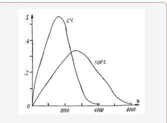
**Figure 5:** Distribution of molecules of hydrogen over their velocities, for two temperatures.
